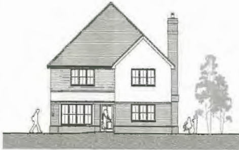
INDICATION ELEVATION OF PLOTS 2 & 4 (PLOT 2 HANDED VERSION) SCALE 1:100
