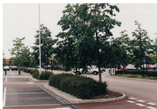
In intensively-used car parks small strips of paving adjacent to parking bays will prevent trampling of planting which results in bare patches
