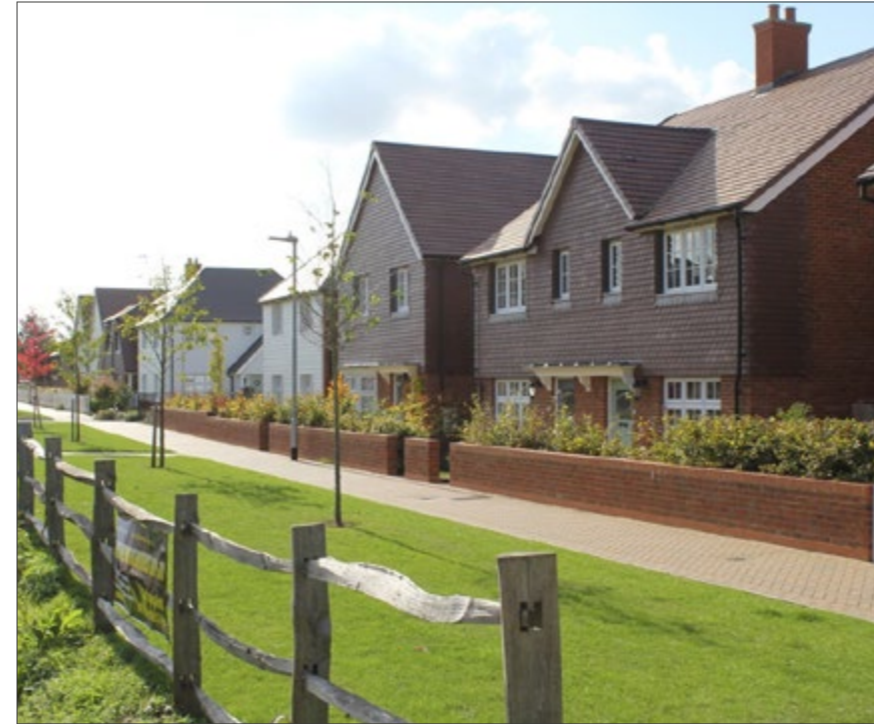
Locally inspired materials: This design uses materials that reflect the locality, such as riven post-and-rail fencing, tile-hanging, and a muted colour palette. Other details such as the consistent boundary treatments, and the swale to within the public realm help add character.
