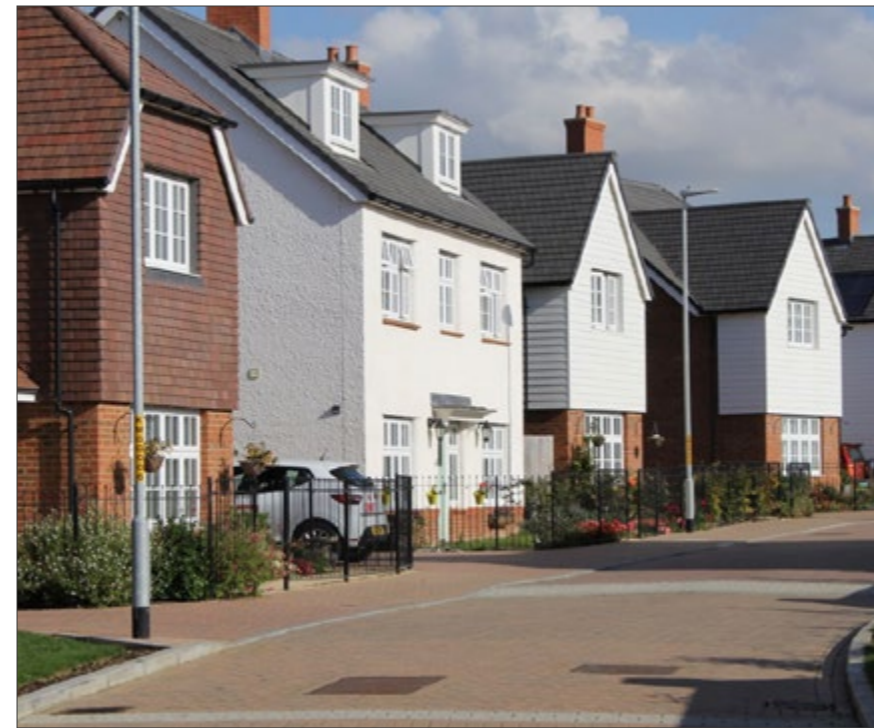
Defining the street: A simple building line, with doors that open to the front, a boundary treatment delineating the extent of the plot, and lots of windows onto the street help to support the usability and attractiveness of this street.
