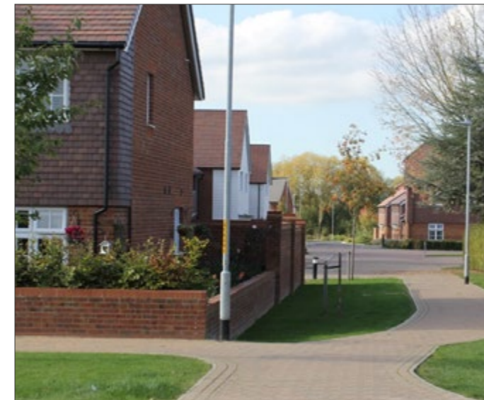
Pedestrian links: This short, well-lit and well-sighted pedestrian link allows people to walk and cycle into and out of the site. Keeping pedestrian and cycle-only routes well-overlooked encourages their use.
