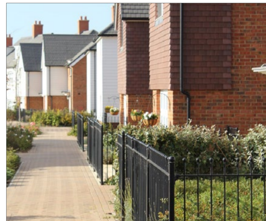
Defining the plot: A simple and consistent boundary treatment helps to mark out what is public and what is private, creating defensible space in front of people's homes.
