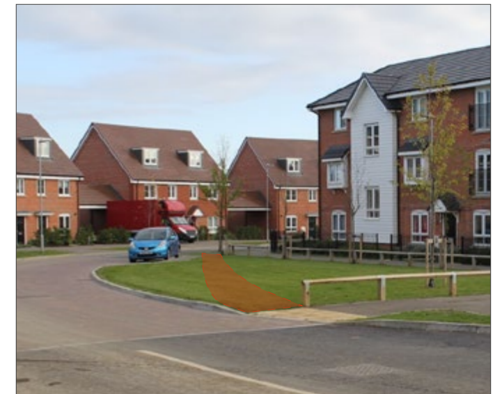
Desire lines: New routes should be aligned so that people can move as directly as possible. Here, the path takes the long route around the green, whereas the quickest and most direct route is partially blocked.
